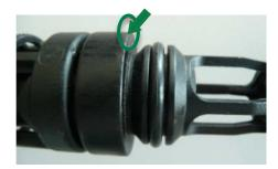
**1** Fix the oil filter element oblique at the edge of the center tube.
