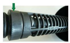
**3** Push the element up to the stop in the housing cover finally, so the two sealing surfaces of the element fits correctly to the center tube.
